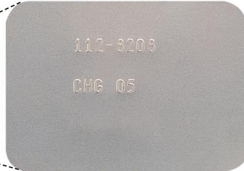
**To ensure you select the right seal kit, locate the cylinder group part number and engineering change level on the outside of the cylinder (example shown here).**
