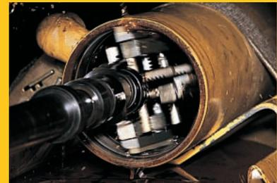
Restoring the proper geometry and surface to the cylinder bore can keep you from replacing seals earlier than necessary. That's why before we install new cylinder seals in our shop we perform a simple procedure called light honing.
