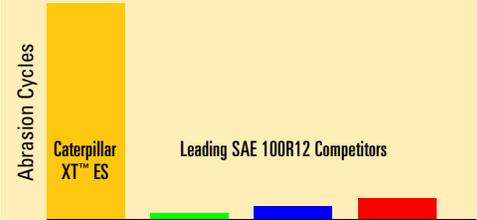
\*\*The International Standards Organization (ISO) abrasion-resistance test requires a 50N (11 lb) steel tool to be cycled back and forth along the length of the hose until the cover wears away to the point of wire exposure.
