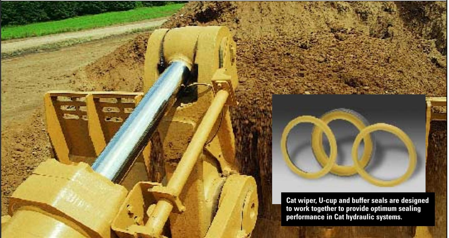
Cat wiper, U-cup and buffer seals are designed to work together to provide optimum sealing performance in Cat hydraulic systems.
