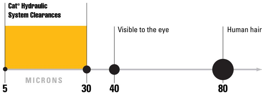
Typical metal-to-metal clearances in Cat® hydraulic systems are 5-30 microns (one micron is one millionth of a meter). Therefore, even particles too small to see can do big damage.
